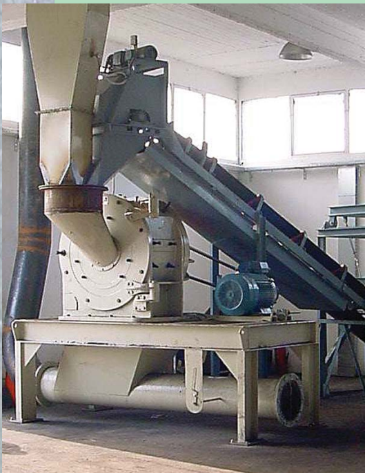
Impact Mill with hot gaz system and pneumatic transport of ground product
